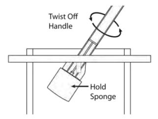
8. Return sampling device to the bag. Do not insert past the thumb stop. Hold sponge from the outside of the bag and twist off the handle by turning counter-clockwise.
