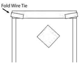
8. Roll down the top of the sample bag several times and fold wire ties over to securely close. Send to a laboratory for analysis.
