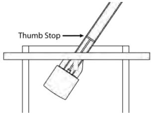
3. Keeping hands outside the bag, guide the handle out the top of the bag. Grasp the handle above the thumb stop and remove the device.
