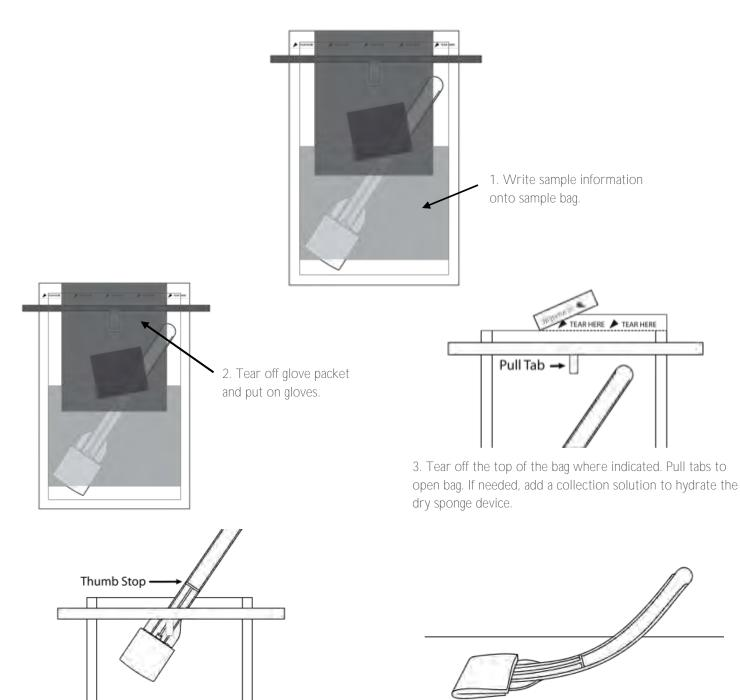
4. Keeping hands outside the bag, guide the handle out the top of the bag. Grasp the handle above the thumb stop and remove the device.
